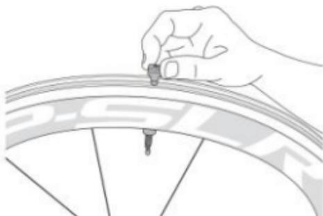
6. Install the tubeless valve onto the rim. The valve nut does not need to be more than finger tightened.
